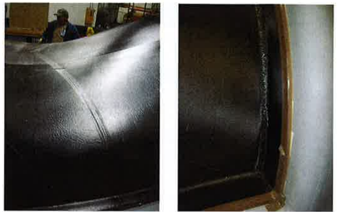
Figure 20. Left - COAD outer monolithic skin after cure showing ply drop region; Right - After cure, the outer monolithic skin had wrinkling in flange radii, particularly in the vertical flange.
