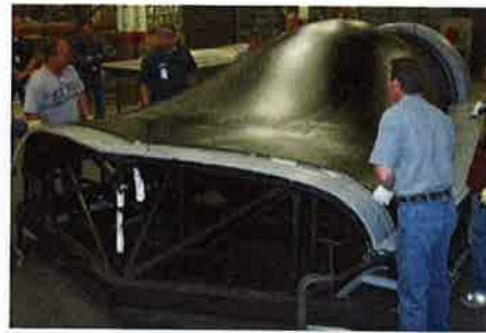
Figure 11. Left - First ply of carbon cloth (MMS 5064, Type 1 – T650/35/5320-1 370gsm 8HS) for monolithic outer COAD skin; SurfaceMaster®905M surfacing film was first applied to the tool before the carbon ply was laid up; Right - After 93°C/12 hour cure, COAD outer monolithic skin is removed from bond jig and put into oven for 177°C/2 hour free-standing post-cure.
