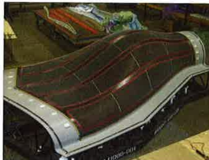
Figure 14. Left - COAD inner honeycomb skin ready for film adhesive and final cloth plies; Right - Lay-up of the cloth prepreg onto FDM tools for co-cured C-channel stiffeners.
