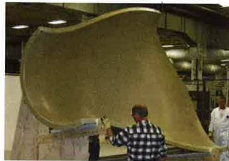
Figure 12. Left - COAD outer monolithic skin after post-cure; placed temporarily back onto Janicki bond jig until AUSS ultrasonic inspection equipment is ready for it; Right - COAD outer monolithic skin loaded onto holding fixtures at AUSS ultrasonic inspection equipment.
