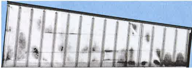
Figure 16. CCPS first skin (cured against Invar tool) ultrasonic C-scan; significant areas of porosity likely due to insufficient pressure caused by lack of thermal expansion of tooling details.
