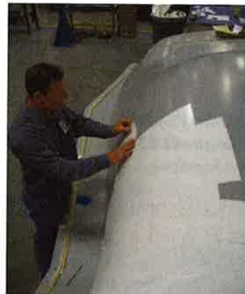
Figure 13. Left - Park Electrochemical Aeroglide™ surfacing film being applied to COAD inner skin tool; Right - Fused deposition modeling (FDM) polycarbonate tooling for co-cured C-channel stiffeners.
