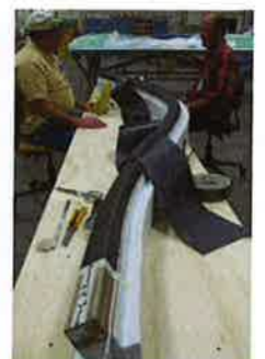
Figure 14. Left - COAD inner honeycomb skin ready for film adhesive and final cloth plies; Right - Lay-up of the cloth prepreg onto FDM tools for co-cured C-channel stiffeners.
