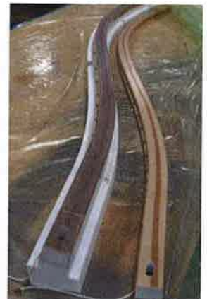
Figure 13. Left - Park Electrochemical Aeroglide™ surfacing film being applied to COAD inner skin tool; Right - Fused deposition modeling (FDM) polycarbonate tooling for co-cured C-channel stiffeners.
