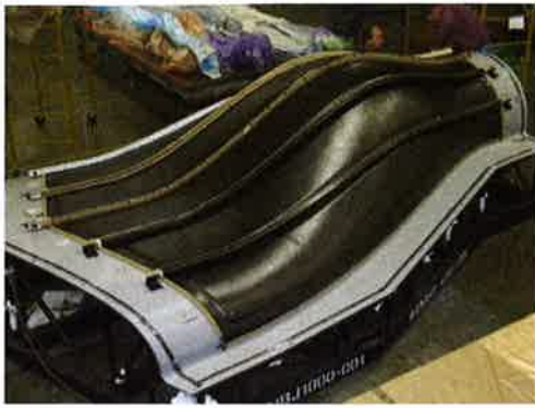
Figure 15. Left - COAD inner honeycomb skin with FDM-tooled C-channels ready for final bag before cure; Right - After cure/post-cure, the inner honeycomb skin is trimmed; outer monolithic skin is in background.
