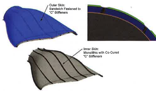
Figure 10. COAD upper half, honeycomb configuration (one honeycomb skin, one co-cured with stiffeners).
