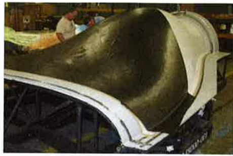
Figure 11. Left - First ply of carbon cloth (MMS 5064, Type 1 – T650/35/5320-1 370gsm 8HS) for monolithic outer COAD skin; SurfaceMaster®905M surfacing film was first applied to the tool before the carbon ply was laid up; Right - After 93°C/12 hour cure, COAD outer monolithic skin is removed from bond jig and put into oven for 177°C/2 hour free-standing post-cure.
