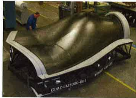
Figure 12. Left - COAD outer monolithic skin after post-cure; placed temporarily back onto Janicki bond jig until AUSS ultrasonic inspection equipment is ready for it; Right - COAD outer monolithic skin loaded onto holding fixtures at AUSS ultrasonic inspection equipment.
