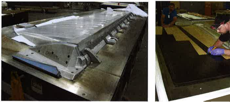
Figure 4. Left – Production tooling consisting of Invar facesheet and aluminum filler blocks; Right – First skin plies being applied (T650/35/5320-1 215gsm unitape).
