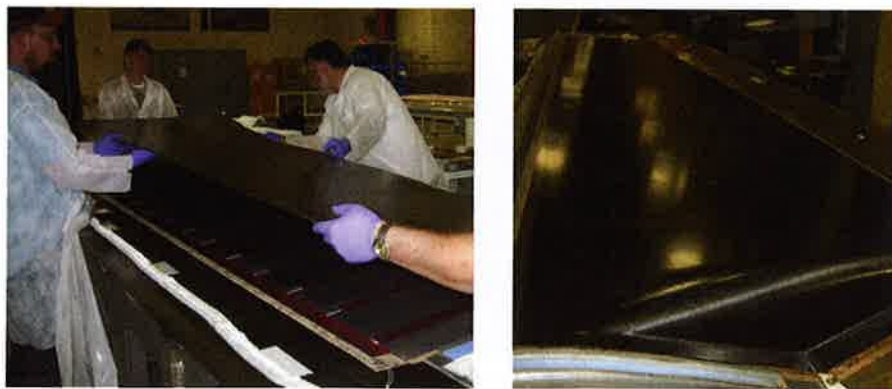
Figure 6. Left – Pre-compacted second skin being applied to filler blocks and uncured composite I-beams; Right – CCPS after cure but before post-cure.
