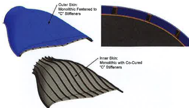
Figure 9. COAD upper half, monolithic configuration (two monolithic skins, one co-cured with stiffeners).
