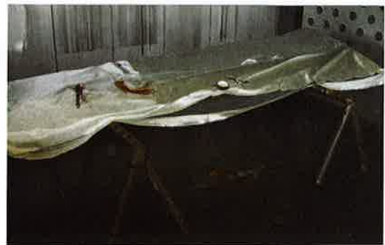
Figure 7. CCPS prepared for free-standing post-cure on very low cost support tooling (metal sawhorses).
