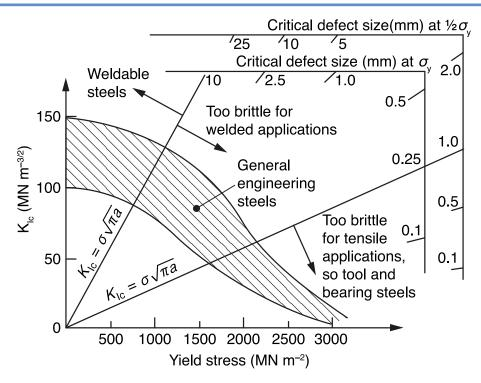
Similarly although very high tensile strength can be achieved in steels by quenching and tempering highly alloyed steels the probability of brittle fracture limits their use in general engineering applications.
