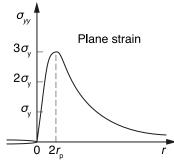
Consider the situation ahead of the crack tip where  $\sigma_1=\sigma_{yy}$  and  $\sigma_2=\sigma_{xx}$  but  $\sigma_{vv}=\sigma_{xx}$ :
