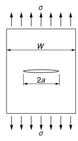
Consider a body containing a crack of half length a and subjected to an externally applied stress,  $\sigma$ . The total energy of the system can be thought of as being the sum of the potential energy term, U plus the surface energy of the crack, S, thus
