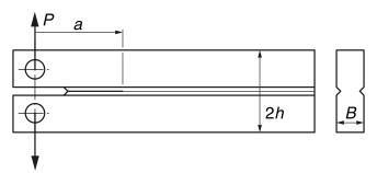
The use of side grooves not only constrains the crack path to follow the midplane of the specimen but also provides more constraint at the crack free surface and thereby promotes plane strain conditions, in principle allowing an overall thinner section to be utilised than would have been the case without side grooves.
