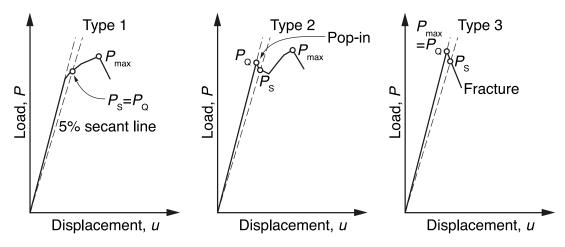
For example if the load-displacement record is of type 1 or 2 then the appropriate load for use in the stress intensity factor expression is found by constructing a secant line with a slope 5% less than the elastic loading line. The intersection of this secant line with the loading line is at PS. If the load at all points on the diagramprior to  $P_S$  is less than  $P_S$  then  $P_S = P_Q$ , as for example in the type 1 record. However if a load point on the diagram prior to  $P_S$  is greater
