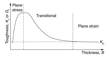
Despite this desire no single test procedure has been developed to allow measurement and interpretation of resulting critical values of *K* or *G* for all possible stress states. Thus, it is customary to consider plane strain fracture toughness testing as the standard methodology and to consider all other stress conditions as exceptions to this standard or requiring a different approach to interpretation of results.
