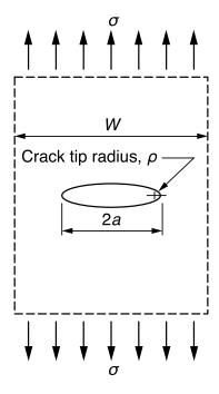
According to a solution due to Inglis the stress at the ends of the crack is given by
