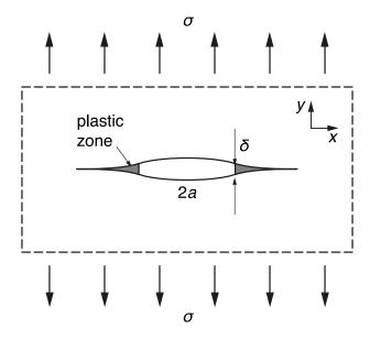
Analysing the Dugdale model and defining the COD as the displacement at the end of the strip yield zone yields the following expression for COD in an infinite plate with a central crack as a function of nominal stress applied,  $\sigma$ , and the crack length a:
