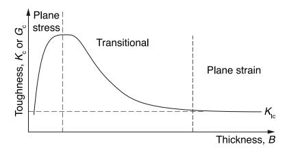
Consider first the plane stress region in which we know from experience that the fracture occurs in a slant plane oriented at proximately 45° to the tensile axis.
