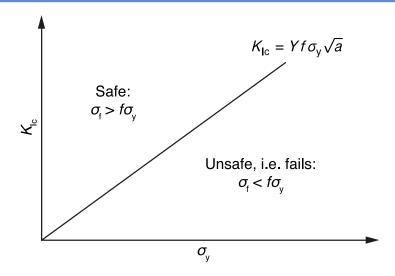
The brittle fracture line divides the diagram into two regions:
