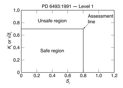
The PD document described in this section evolved to become a FAD-type method. In its first version (1980) PD 6493 proposed the fracture assessment in terms of the COD design curves. It consisted of a **design code**, in the sense that not only was a fracture assessment line proposed (i.e, the relationships themselves), but a whole set of assessment guidelines was given. The 1980 version included assessment against fracture, fatigue, overload, leakage, creep, buckling and environment effects.
