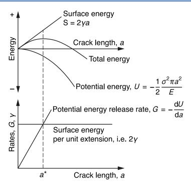
Fracture is deemed to occur when the potential energy release rate, G exceeds the surface energy per unit crack extension which must be provided to the system if crack growth is to occur. Where these two lines meet the crack length is the **critical** or **Griffith crack length**,  $a^*$ .
