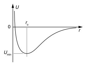
What we want to know is the magnitude of the force and hence the stress required to cause a crystalline solid to fracture across a particular crystallographic plane. To carry out such a calculation we need to consider each atomic bond as a spring element initially at a separation of  $r_0$ .
