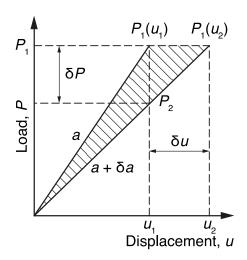
As the crack extends the stiffness of the plate will decrease such that because the grips are fixed (equivalent to fixed displacement, i.e. constant  $u_1$ ) the load applied by the grips will decrease as the crack extends. In energy terms we can see that for crack length a the elastic strain energy is given by  $\frac{1}{2}P_1u_1$  and that this changes to  $\frac{1}{2}P_2u_1$  as the crack extends to  $a+\delta a$ .
