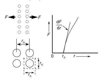
If the bond is stretched to the max value  $F_{\rm m}$  of F, it will be unstable and will break if the stress continues to increase. Therefore an estimate of the tensile strength could be obtained by calculating  $F_{\rm m}$ . However instead of considering the maximum force  $F_{\rm m}$  we can arrive at a value for the maximum stress directly by making the connection that each atom effectively occupies an area of  $r_0^2$ .
