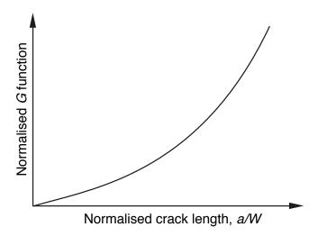
Having successfully determined the compliance function for a particular geometry an energy release rate function can then be derived as a function of crack length which can be used to calculate  $G_{\rm c}$  (the critical value of strain energy release rate or "fracture toughness") in subsequent tests using specimens of the same geometry.
