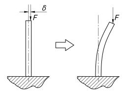
Jamming can occur when, as a result of an oversight in design, excessively large elastic deflections take place. It is a risk in the design of engines, for example, when clearances between components are very small.
