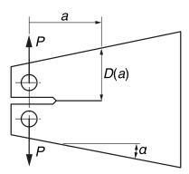
This specimen geometry with an angle  $\alpha$  of about 12° gives a reasonably constant K over the central section of the specimen but is not truly constant. This type of specimen geometry is most frequently employed when fatigue crack growth rate or environmentally assisted crack growth rate data has to be determined.
