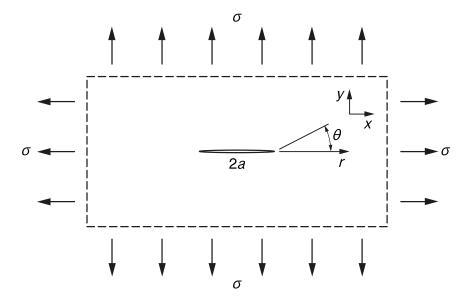
Defining a cylindrical coordinate system with the origin at the tip of the crack, the stresses can be written as a function of the radial distance, r, and the angle,  $\theta$ :
