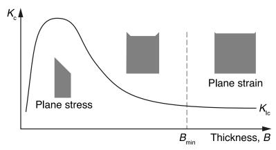
Above a certain thickness  $B_{\min}$ , the fracture toughness has a minimum value which is independent of thickness. This minimum value of  $K_{\text{c}}$  is known as the plane strain fracture toughness and is denoted by  $K_{\text{lc}}$ . Particular attention is paid to  $K_{\text{lc}}$  because this is the minimum toughness that can be achieved under the most severe conditions of loading.
