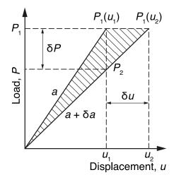
We know that the strain or potential energy release for an increment of crack growth  $\delta a$  is given by  $G\delta a$  per unit thickness and if we define B as the thickness of the plate we can say that:
