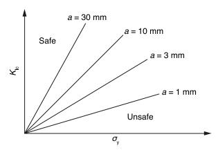
For a particular crack length any combination of fracture toughness and applied stress which puts us to the left of a line implies a 'safe' condition whereas any combination which is mapped to the right of a line implies a potentially 'unsafe' condition. Hence for a particular crack length, the critical failure stress can be easily determined or, for a particular applied stress, the maximum tolerable defect size can be determined.
