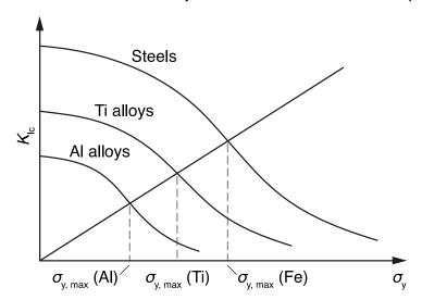
Having identified the highest usable strengths, can then calculate required section sizes and compare weights, costs, etc..
